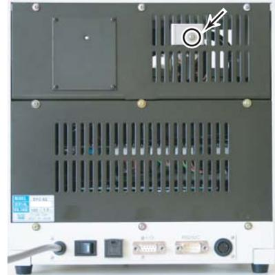
**Fig. 1** Unscrew and pull the fixer.
