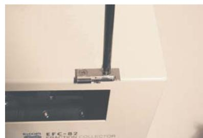
**Fig. 8** Fixing the hood.
