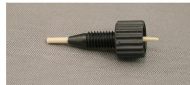
Keep the flat end of needle out from the tip of screw while tightening Easyfit screw. After fixing Easyfit Screw, the length of tubing sticking out inside of port will be 1 to 2 mm. If you tightened hard and then unscrew Easyfit, you can see how much the needle is projecting inside.
