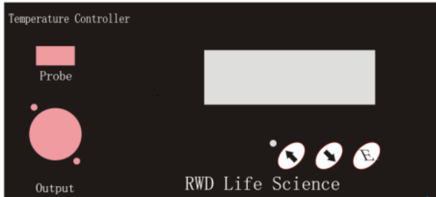
Fig.4 the front panel of the Control Unit
